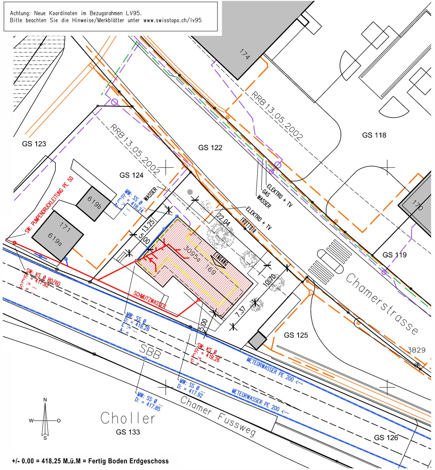
+/- 0.00 = 418.25 M.ü.M = Fertig Boden Erdgeschoss
